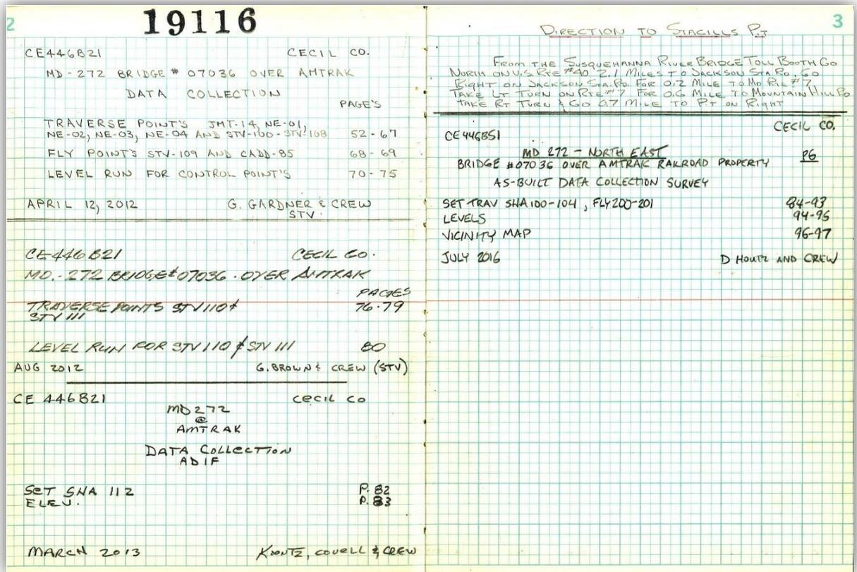
vi. Index notes for GPS work shall include control points set and control points used.
