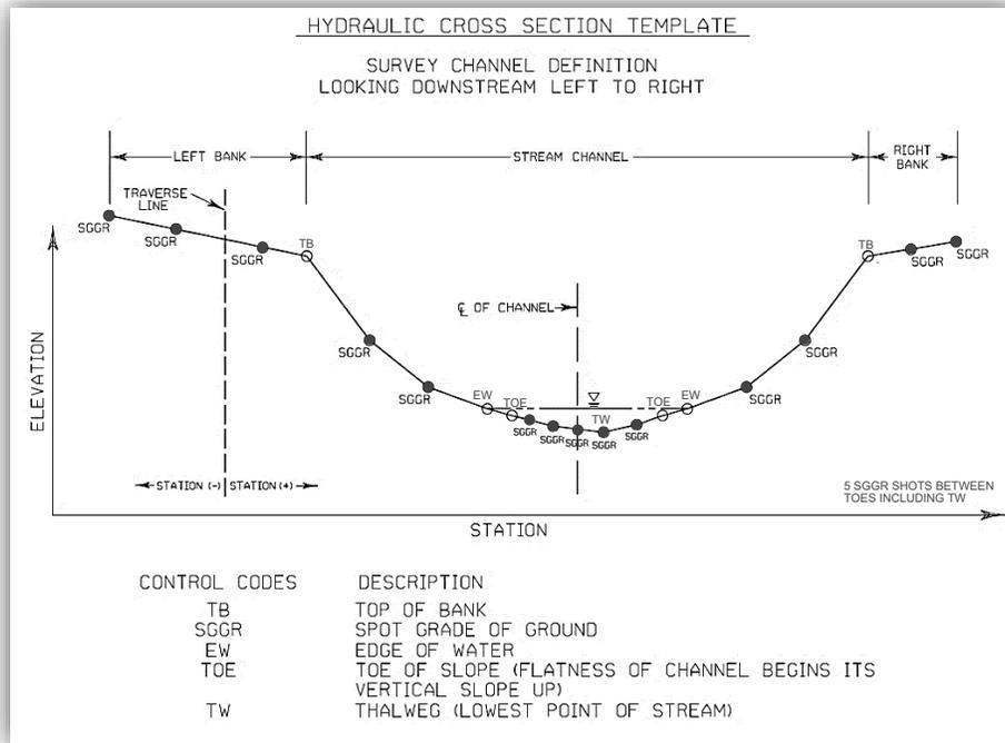
ix. Some cross-section requests will require profiles to be collected in the same manner for the road surface over a structure or bridge.
