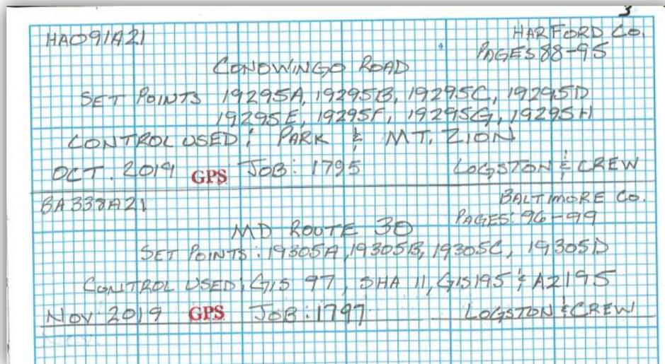
vii. For each new RTK traverse point set, bookwork must be performed to document the establishment of the control point. The following details shall be included as shown below in the example. This bookwork must to be done in addition to filling out the RTK Observation Logs as shown in [section 9.E](#).
